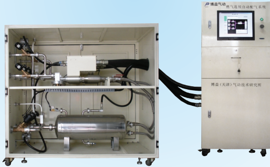
燃气连续自动配气系统 Gas Continuing Automatic Mixing and Distribution System
