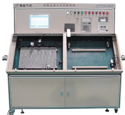
散热器气密测试装置 Radiator leak testing device
