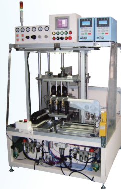
进排气歧管气密测试装置 Intake-exhaust manifold Leak testing device
